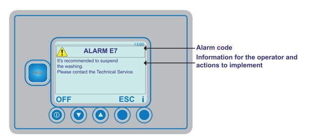
If the alarm does not block the machine it is possible to continue the operation by pressing **6 ESC** key. The machine will continue to signal the alarm until the resolution of the problem by:
