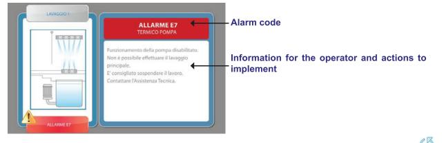
If the alarm does not block the machine it is possible to continue the operation by pressing **RETURN** <sup>(U)</sup>. The machine will continue to signal the alarm until the resolution of the problem by:
